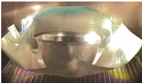
Image 2: Active air removal (pack expands)
